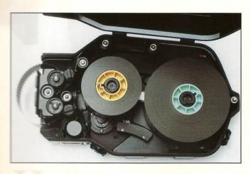
A true displacement magazine, the shaft of each film roll shifts progressively as the film is exposed. This reduced weight shift makes the AATON 35-II ideal for Steadicam® operation.
